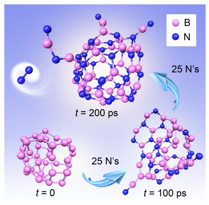
Quantum chemical molecular dynamics simulation of boron nitride fullerene formation from an amorphous boron cluster.
